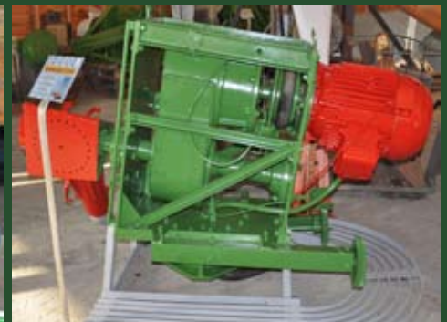
Blacksmith's 22kW nacelle
